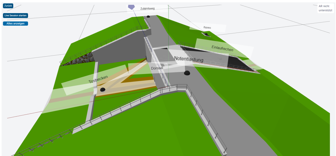
Figure 39: Bottom outlet of a retention basin made by students
