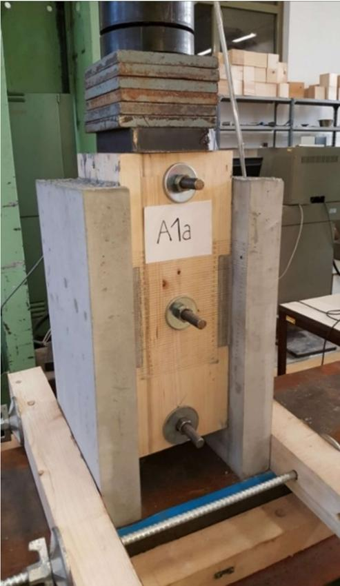
steel-concrete composite specimens
