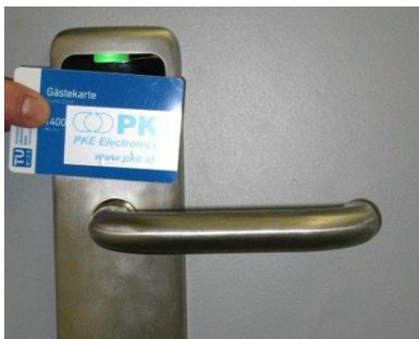
To activate the Office function, the card must be held against the reader until two optical/acoustic signals are visible. The door can be opened without using the card.
