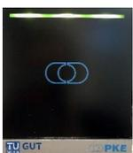
Three bright green LED lights shining mean that the door can be opened without using a card.
