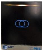
If an orange LED light indicates in the middle, the card has been removed too quickly from the card reader and the permissions could not have been transferred to the card. Hold the card to the card reader again until 3 LED lights light up green again; the door can be now opened.
