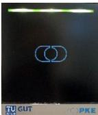
If all 3 LEDs light up bright green and a beep is sounded, the transfer of offline authorisations is completed and the door lock is released for a single door opening.
