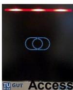
The red LED light blinks and the card is rejected. The lock on the door is not released and the door cannot be opened. (Causes: missing access authorisations expired TUCard (visible at the back of the TUCard - "Valid to" date).
