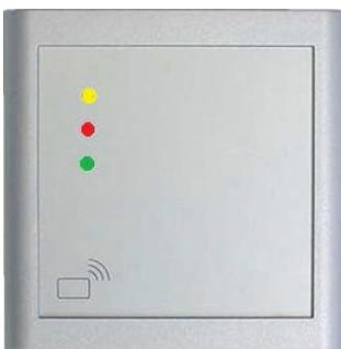
The red and green LED lights blink alternately during the booking process. After successful description of the card, the green LED light turns on and a beep is sounded from the card reader. After that, the door lock is released and the door can be opened.
