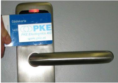
Red flashing LED light means that the card has no authorisation and therefore the door cannot be opened.
