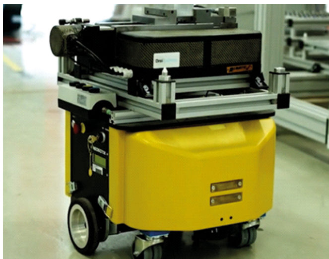
autonomous material handling of the 5G-machine vice (at time of photo still a prototype) in a production facility
