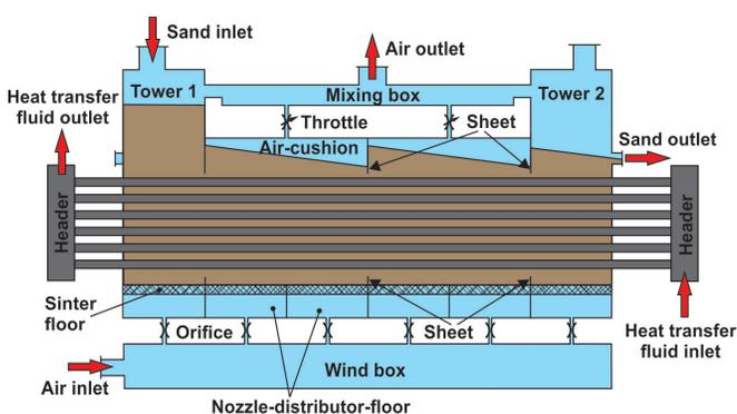
Scheme of the SandTES heat exchanger
