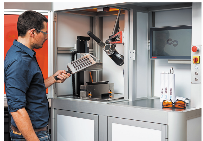
Hot Lithography production machine for highly viscous photopolymers
