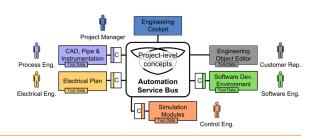
The effort for building quality assured tool chains from heterogeneous software tools from several disciplines should be reduced. The data exchange standard AutomationML (AML) and the integration platform "Automation Service Bus®" together enable the project team to achieve this goal.
