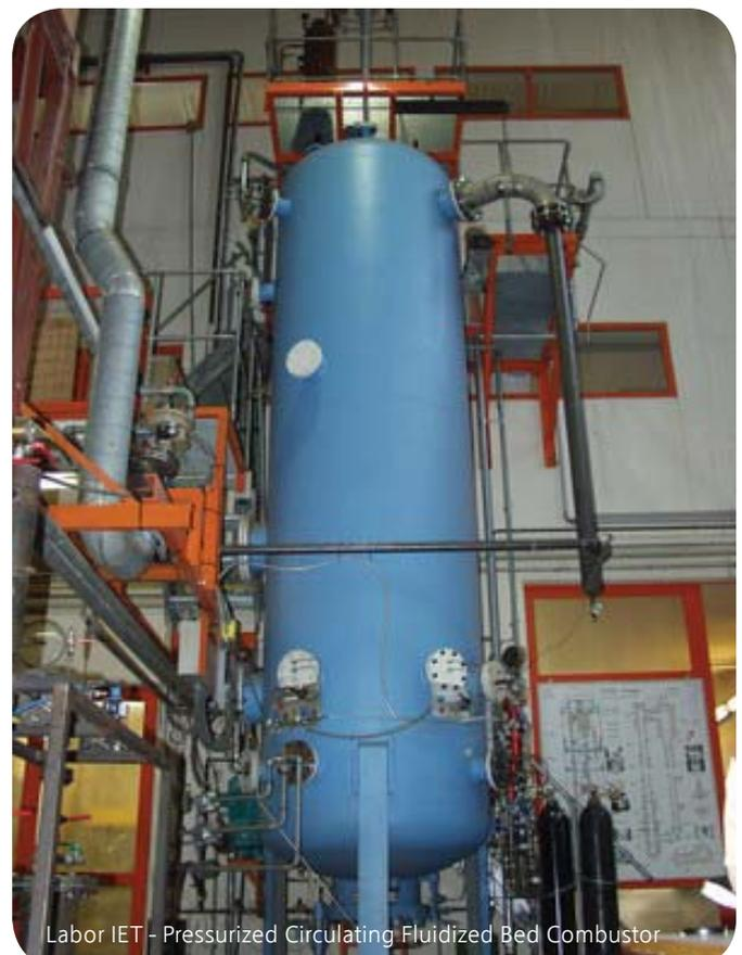
Labor IET - Pressurized Circulating Fluidized Bed Combustor
