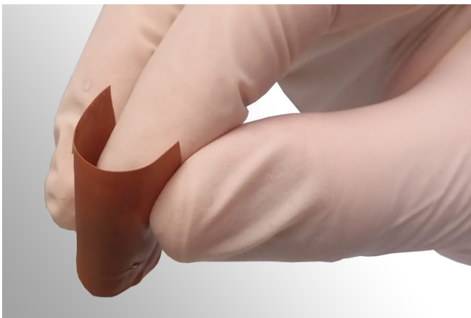
A composite film reinforced with CRYS particles showing high thermal and chemical stability combined with flexibility.
