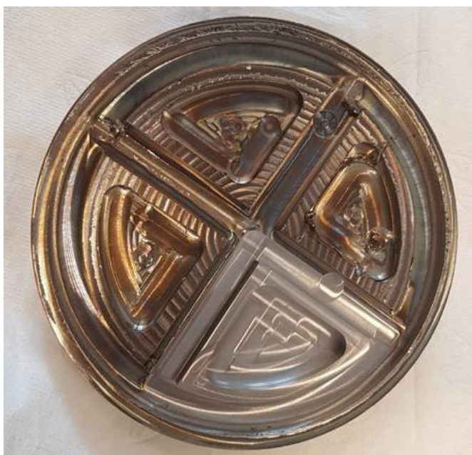
High-speed machining of Inconel 718 Precision part with sophisticated geometry – one sector after finishing operation
