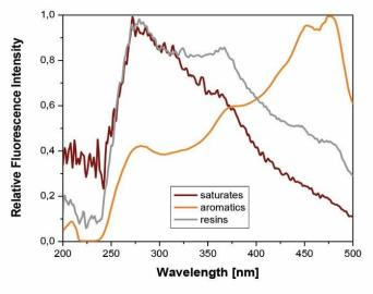
Typical spectral lines of bitumen's essential components
