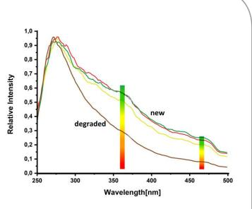
Fluorescence spectra of bitumen of different road surfaces
