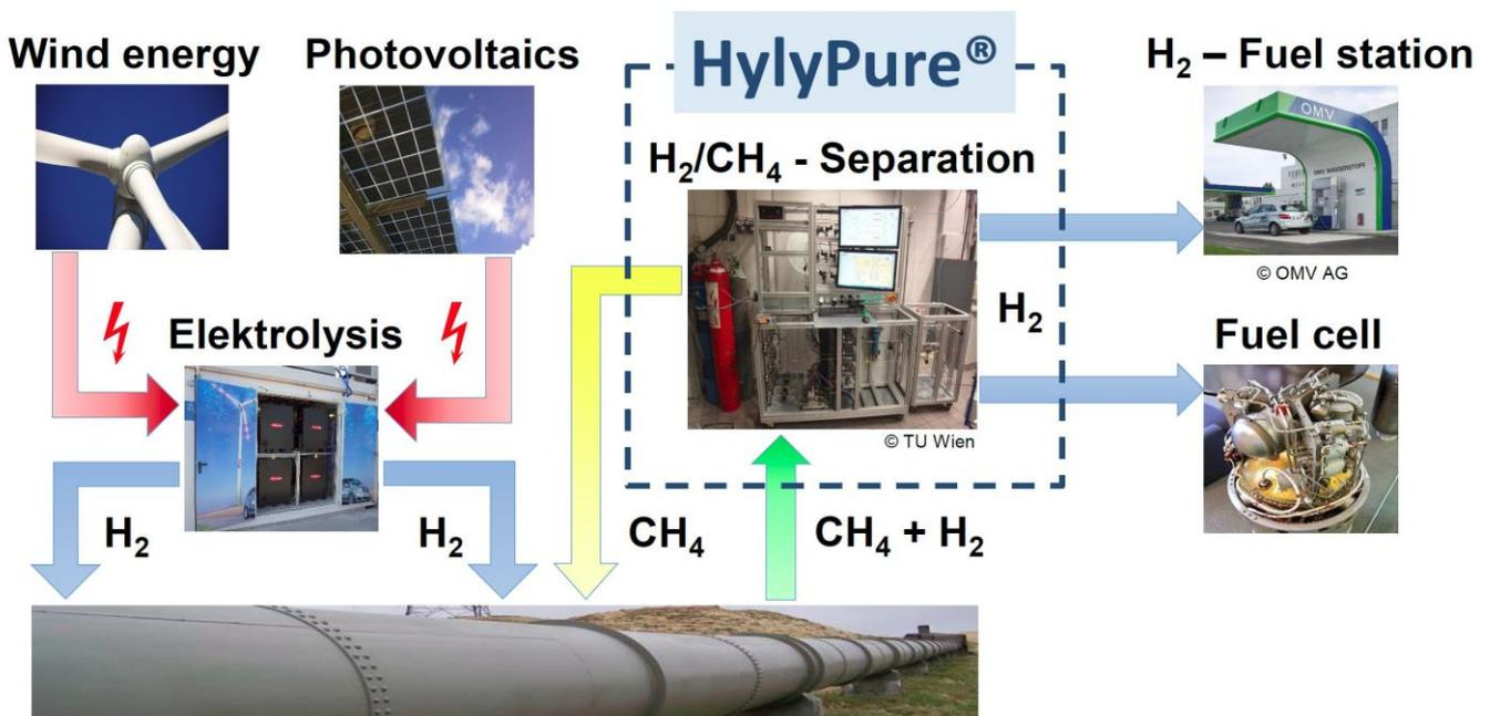
Supply of green hydrogen by means of HylyPure<sup>®</sup>
