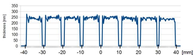
Thickness-distribution of P3HT:PCBM-strips on PET
