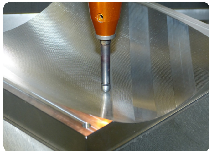
Functionalising a surface via automated hammering
