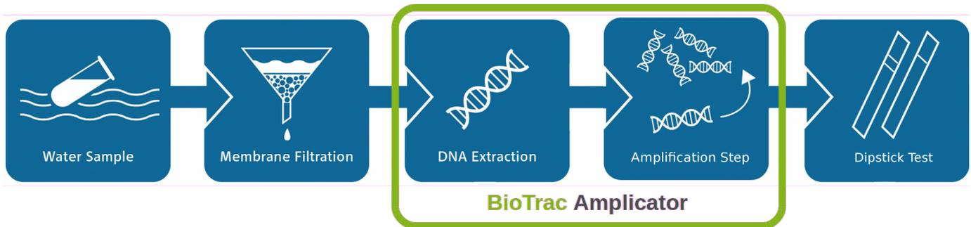
The Amplicator, which enables the rapid, straightforward detection of the contamination, was developed in cooperation with BioTrac. All that is needed is a small analysis device in combination with special reagents in order to multiply the specific DNA traces. An evaluation of the results takes place with straightforward test strips of the type that is known from pregnancy tests. With the new Amplicator, the entire analysis time, from the sampling to the result, takes just three hours.
