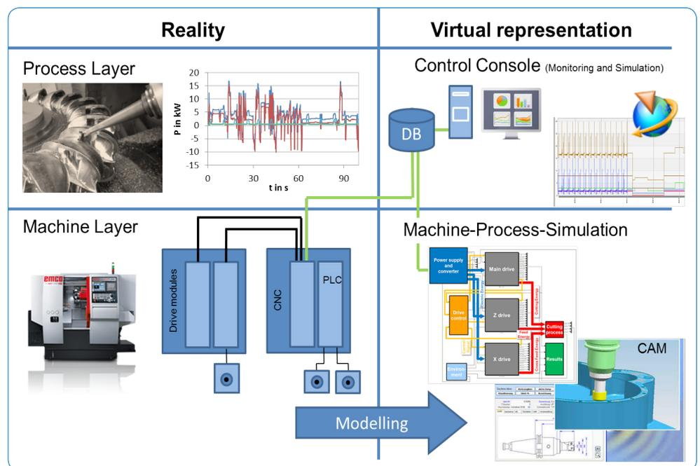
Concept for utilisation of energy and control data for optimisation of manufacturing control
