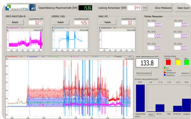
Visualization of the energy monitoring of a machine shop
