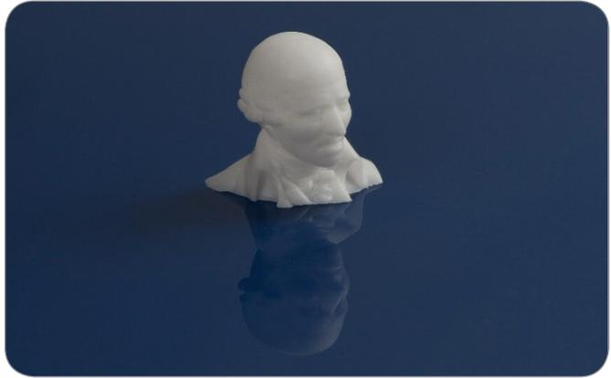
Joseph Haydn – 3D printed, made from Al<sub>2</sub>O<sub>3</sub>
