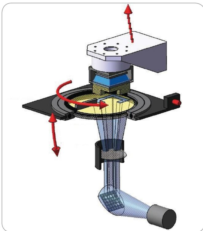
3D printer developed by TU Wien (principle scheme)
