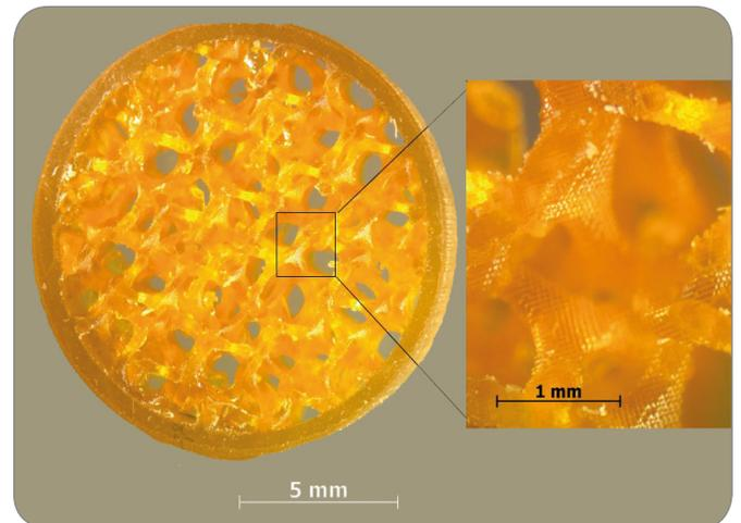
3D printed cellular polymer structure
