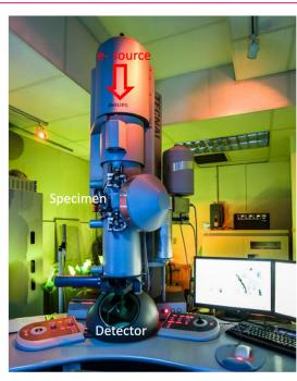
**FIGURE (above):** Spin resonance spectroscopy with a transmission electron microscope ©TU Wien
