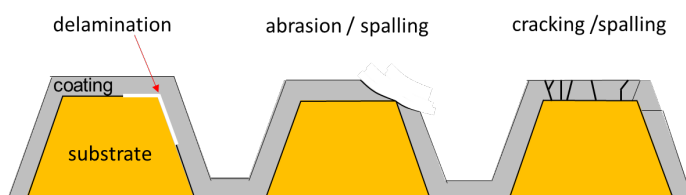
Image 3: Schematic of possible types of failure in coated samples © TU Wien
