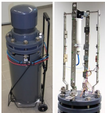
MICRA-buoy 1 and its integrated sample holder
