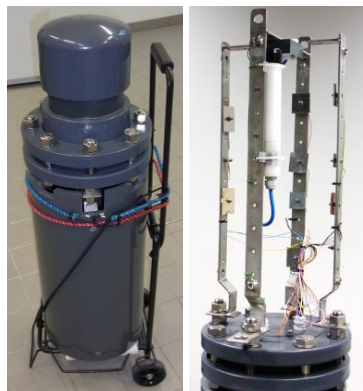
MICRA-buoy 1 and its integrated sample holder
