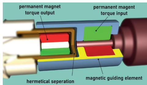
Fig 1: cross-sectional-view of the miniature magnetic coupling
