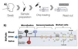
The newly developed microfluidic device consists of 4 parts: microfluidic channels, nanosensors. readout. and microbatteries for power generation. The novel nanobiosensing strategy allows rapid, reliable and accurate detection of viruses and
