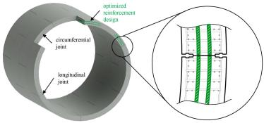
Left: Segmental tunnel lining structure. Right: Detail of the optimized reinforcement design in the longitudinal joint.
