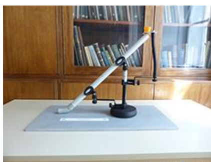
Figs.: Prototype of the TU Wien floor slip tester with a height of about 20 cm. The pattern of scattered material shows the slip resistance class of the floor.
