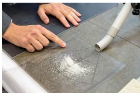
Figs.: Prototype of the TU Wien floor slip tester with a height of about 20 cm. The pattern of scattered material shows the slip resistance class of the floor.
