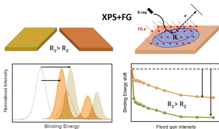
From metals over semi-metal towards differently doped semiconductor type materials it was found that recorded shifts of XPS signals of the ionic liquid correlate not only with flood gun intensity, but also with charge carrier concentration of the solid underneath [1, 2]. Thus, this method represents an alternative way if compared to state-of-the-art methods and may be of interest not only for bulk type materials, but also for thin films, multilayer or 2D materials
