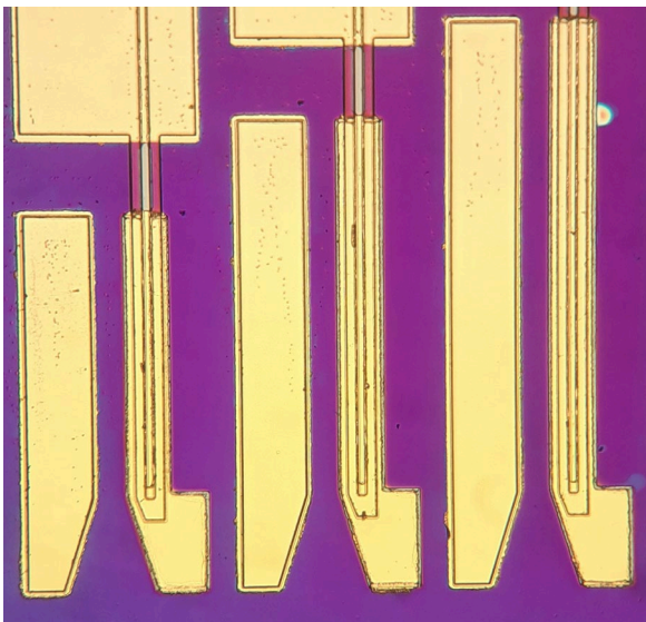
Microscope image of an interband cascade laser frequency comb chip with optimized radio-frequency injection contacts.
