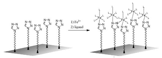
Figure 1: Top-down approach for self-assembly of spin crossover monolayers
