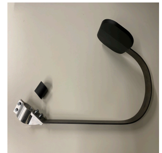
Prototypes of the support device: 3D printed (left), made of spring steel featuring an adapter for different saddle tubes (right)
