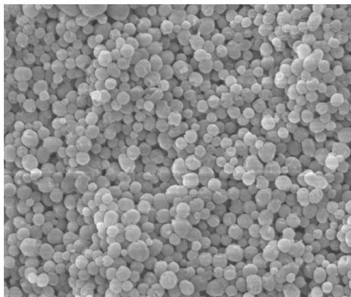
The received lignin nanoparticles are in the range of several 100 nanometers and can be influenced by the extraction and the precipitation parameters. The produced nanoparticles can be derived in uniform particle size distribution as can be seen in the picture.
