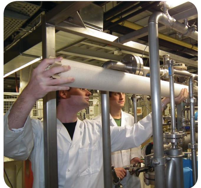
Three-stage pilot system (RO/NF/NF) with five 4" membrane modules
