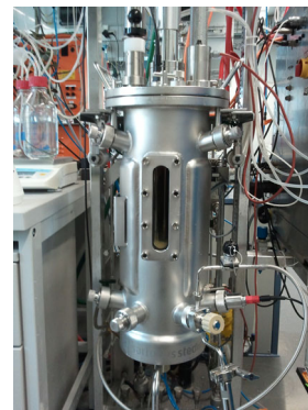
Fig. 1: Bioreactor for biological methanogenesis process
