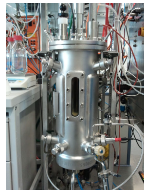
Fig. 1: Bioreactor for biological methanogenesis process
