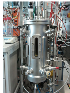
Fig. 1: Bioreactor for biological methanogenesis process
