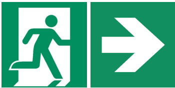
Figure 2: E002 Emergency exit (right) as per ISO 7010:2012 and arrow type D according to ISO 3864-3:2012
