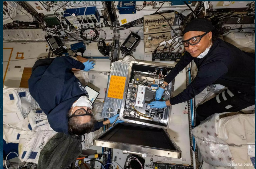
Removal of Metal 3D from EDR2, printed specimen A retrieval, printer health checks, new build plate installation, printer back in EDR2 for next print ISS astronauts Jeanette Epps and Sunita Williams (21 st Aug 2024)
