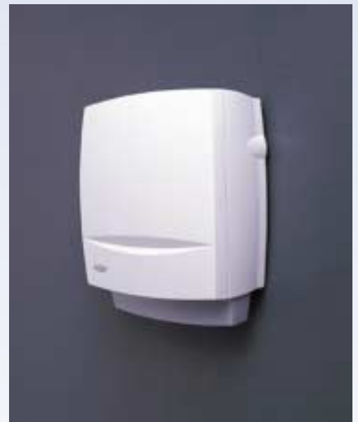
The MCellarena Base Station from MOTOROLA provides targeted high capacity, high quality coverage in areas of high
