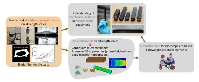
This thesis will contribute to the mechanical identification of fiber-level properties (left), which will be used as input for advanced multiscale simulation approaches (middle, bottom) to develop 3D material models for biocomposite elements (right) and improve the understanding of the mechanical behavior of this new type of material (top).
