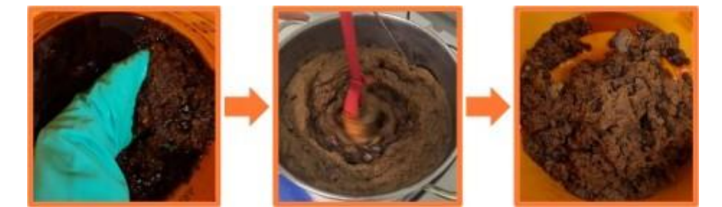
Figure 2. Impregnation of the produced fibers and solvent removal to prepare the sample to be pressed.
